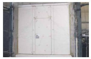
To determine the fire protection class, one wall face of the Variflex EI 30 with integrated pass door was exposed in a test laboratory to the direct flame of a test fire for half an hour.
