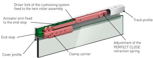
Inside Portavant 150, the proven design principle of the Portavant series ensures outstanding quality and technology:
